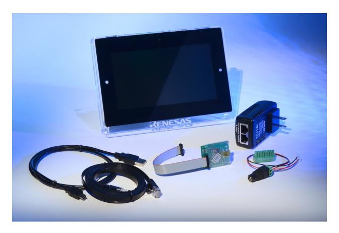
The PE-HMI1 also includes an external J-Link lite debugger.
